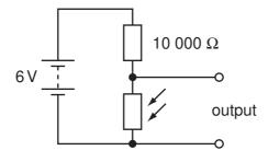
What should be the resistance of the LDR for the output to be 3V?
